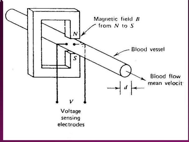
The volume of blood Q through the vessel can then be calculated.
