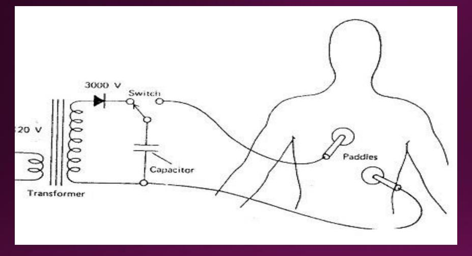
Fig. 4). A simple defibrillator. The line voltage is stepped up to several thousand volts by a transformer. A diode rectifies the alternating current into direct current to charge up the capacitor. When the switch is thrown. The capacitor discharge through the paddles and the heart.
