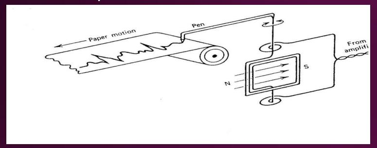
After amplification, the ECG signal must be displayed. When a routine diagnostic ECG is taken, a permanent record is required for analysis and a pen recorder is usually used (Fig.3). In a pen recorder, the amplifier output passes through a coil of wire suspended in a magnetic field. In the same way that a galvanometer twists when current passes through it, the pen twists to write on a moving strip of paper.
