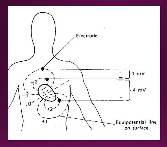
Fig.2. The dashed lines show the resulting surface potentials. The difference in the measured potentials caused by using different electrode locations. Both voltage and polarity my change with electrode position
